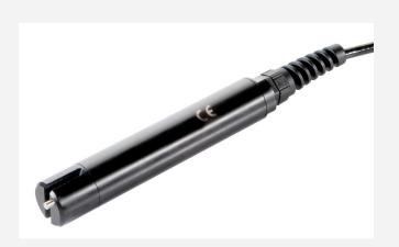
The conductivity probe utilizes four electrodes; two made of graphite and two made of platinum. The possible applications of this sensor range from freshwater to surface water and all the way to municipal and industrial wastewater.
